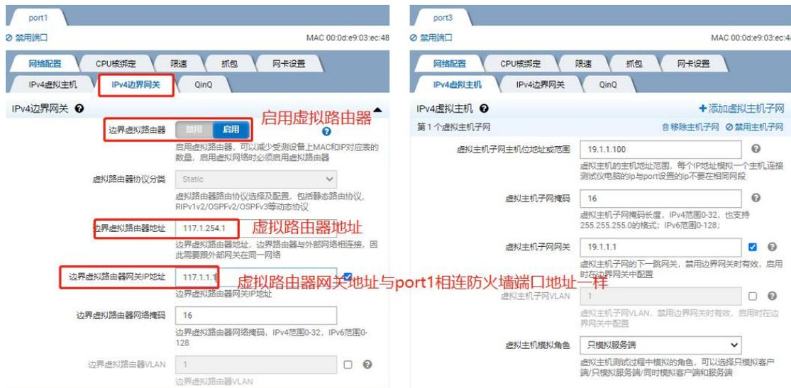
The screenshot shows the 'IPv4边界网关' (IPv4 Boundary Gateway) configuration panel for the client. The '启用' (Enable) checkbox is checked.
